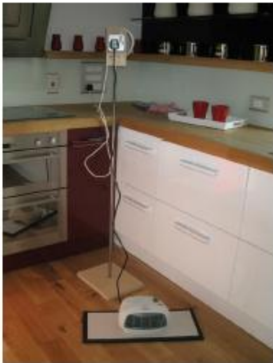
Figure 2.1: Thermostatically controlled Fan heater used in Co-heating test
