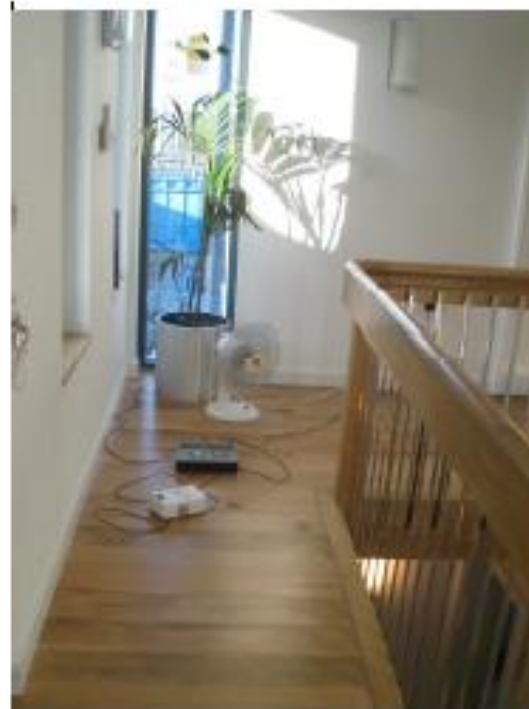
Figure 2.2: Pyranometers and data logger being installed for Co-heating test
