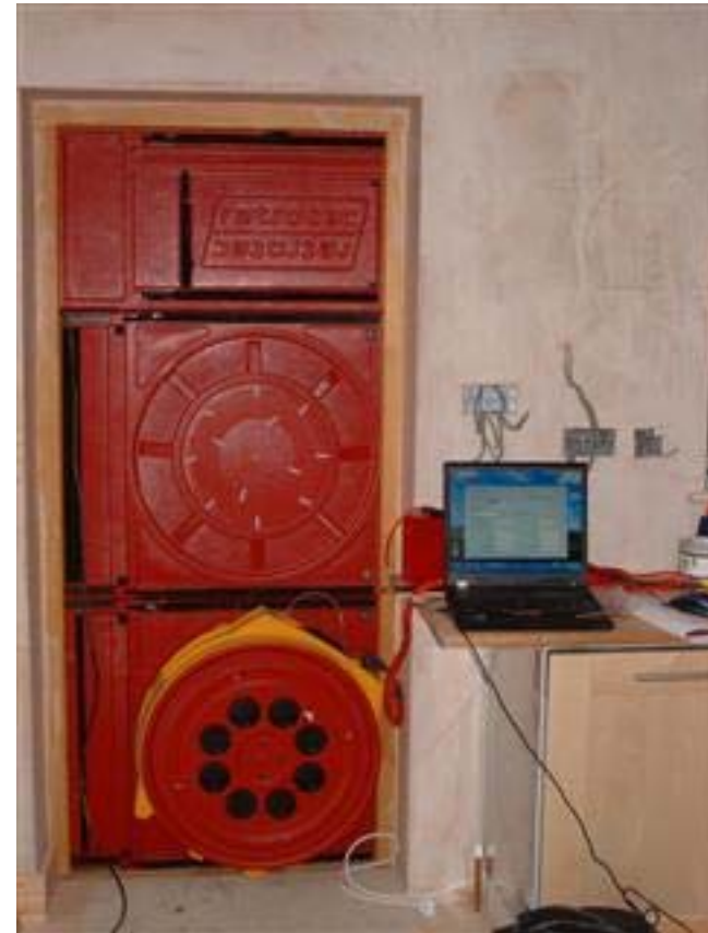
Single fan kit mounted in a doorway testing a low-energy house near Oxford
